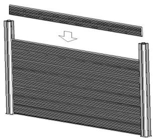
\*only use the board separator (A) to create spacing between the horizontal boards
